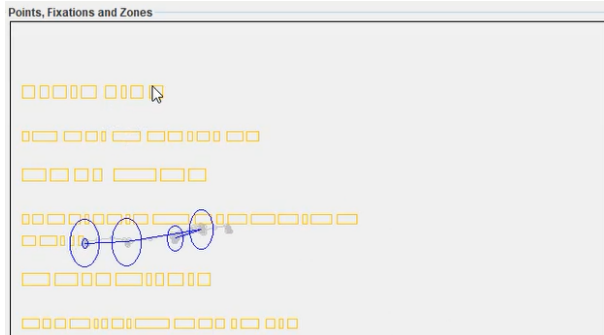
Figure 2: Eye tracking data visualization with Zones (yellow rectangles), Gaze Positions (grey points), and Fixations (blue circles)
